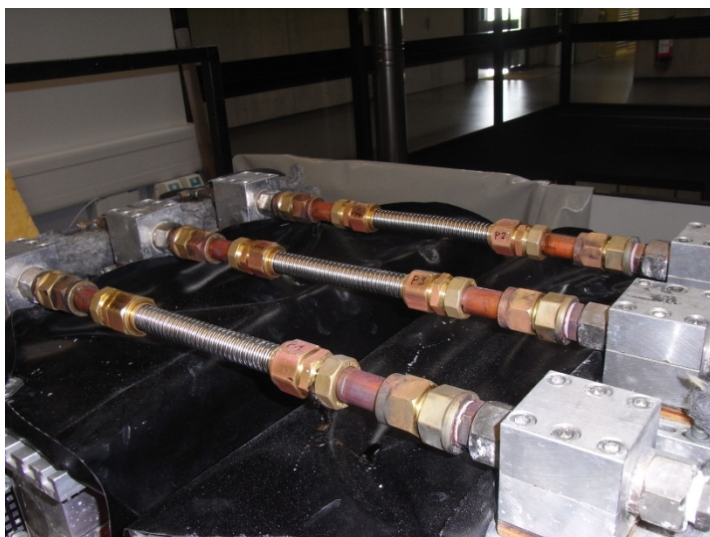
Figure 6: (after test) Samples installed on the test rig. No leakage or any other problems have been observed.
